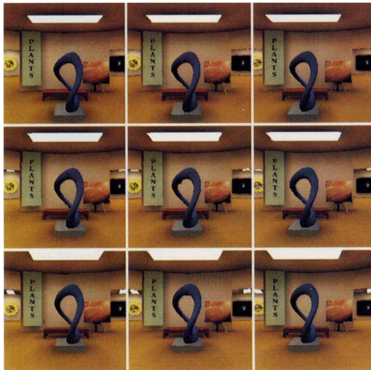
Fig. 10 2D interpolation. The source images are in the corners. All the other images are interpolated from their nearest three source images. (The center one is interpolated from the upper two and the lower left corners.)
