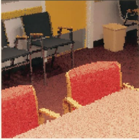
Fig. 10. A low-resolution, rectangle-filled quadtree rendering of a conference room.
