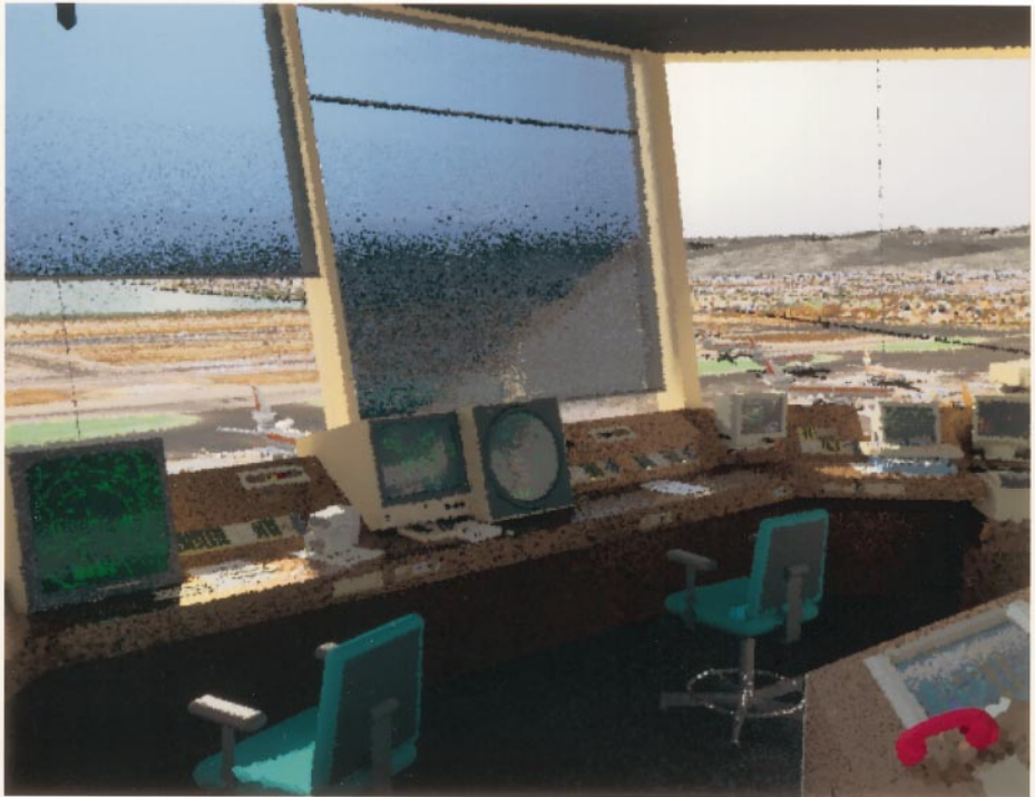
Fig. 33. The same simulation after 30 seconds of progressive ray tracing on 21 processors.
